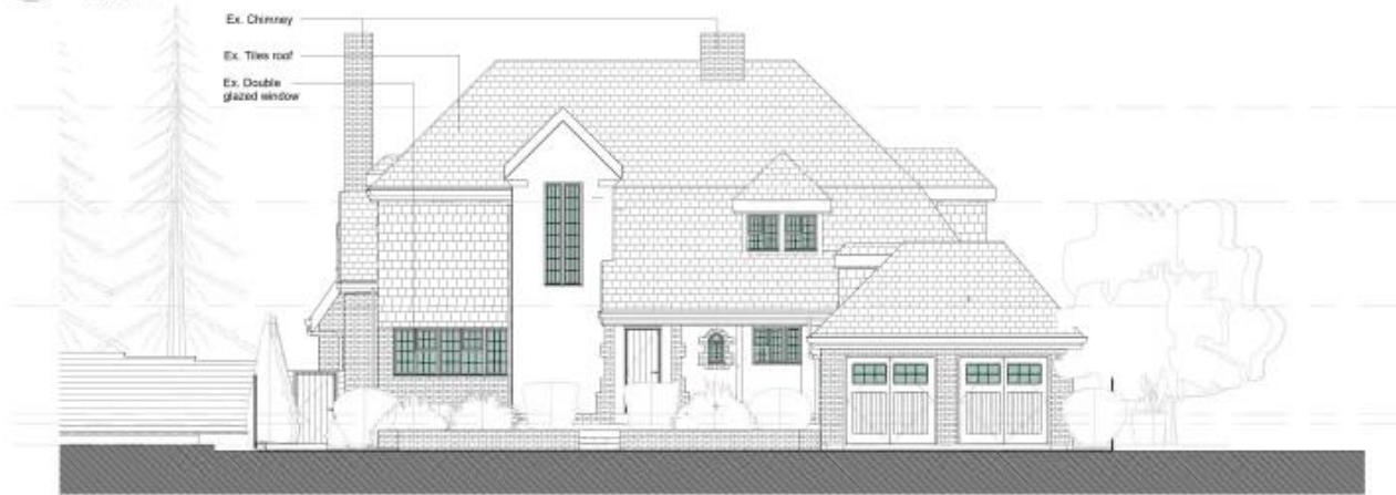
4 Existing Elevation - South 1 : 100
